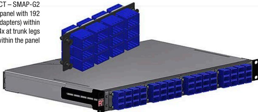
Figura 3 – 400GBASE-SR8 PreCONNECT – SMAP-G2 HD 19" 1 HU 3/3 panel with 144 (36 MDC4x adapters) within the patch field, 2 PreCONNECT SEDECIM MTP 16F interfaces per cassette back plane
